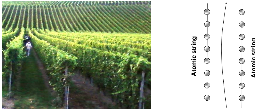
Figure 1. Left: A colorful way to demonstrate channeling. Picture captured by one of us (H.B.) at the vineyard Baiken at Rauenthal, Rheingau, Germany. Right: Channeling of a positively charged particle. Shown are two strings of atoms composing crystal planes.
