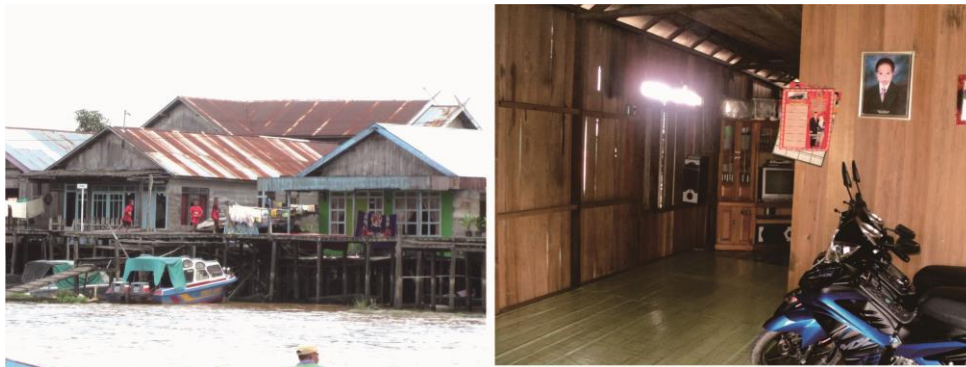
Figure 9. The use of zinc as a roof cover (left) wooden board as a ceiling to reduce heat (right)
