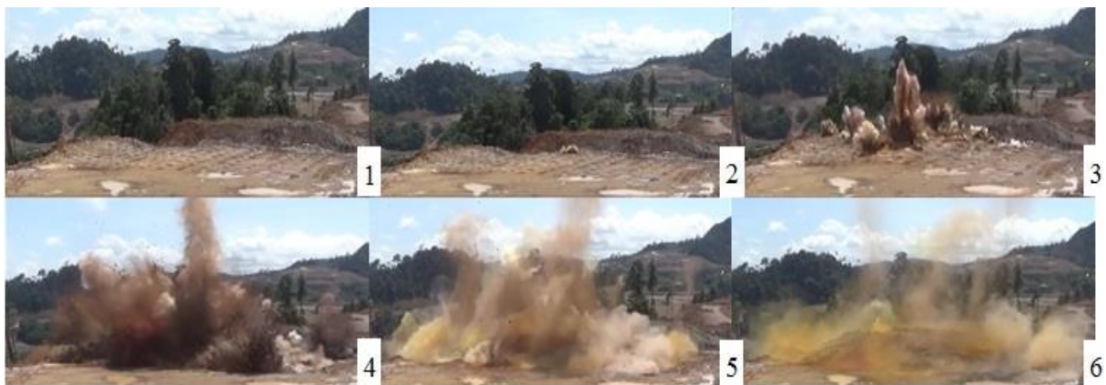
Figure 5. View of The Detonation Sequence of Bench Blast at Martabe Project (Type:BPM)
