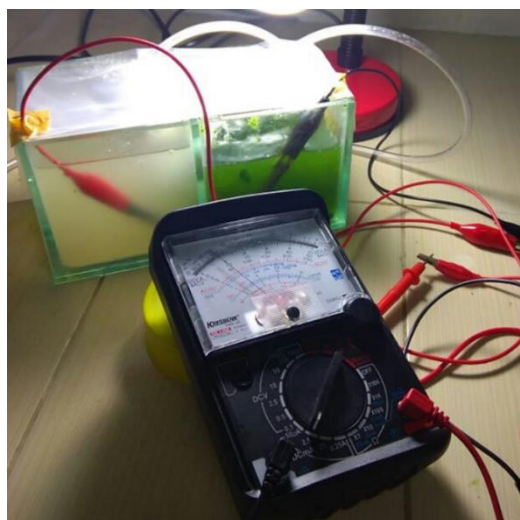
Figure 1. Photograph of MMFC configuration.
