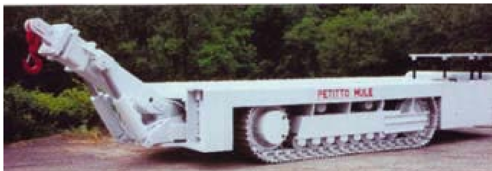
Figure 2. Machine Petitto Mule model 1550 is designed to extract support sections with a mass up to 36 tonnes.
