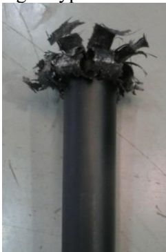
(b) Tearing of type B carbon fiber
