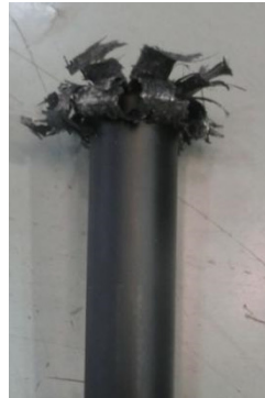
(a) Tearing of type A carbon fiber
