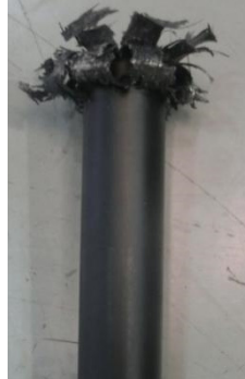
(c) Tearing of type C carbon fiber
