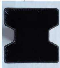
Figure 12. Sectional view of the polygonal square tube
