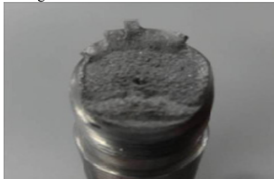
Figure 6. Macrograph of vertical link fracture.
