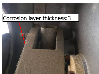
Figure 2. Macroscopic picture of No.510 connecting lever.
