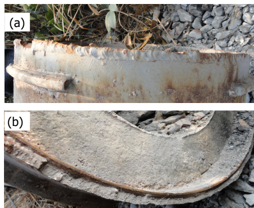
Figure 6. (a) Side view of upper weld crack, (b) Top view of upper weld crack.
