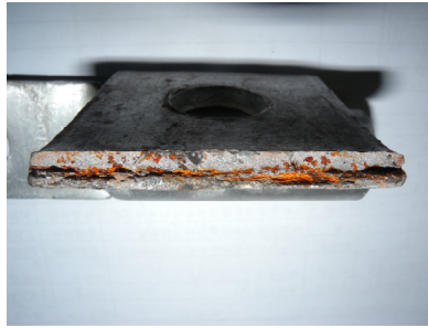
Figure 2. Fracture appearance of hoop.
