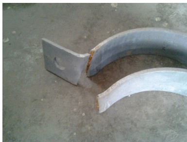
Figure 1. Scene photograph of cracked hoop.
