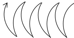
Figure 6. A schematic diagram of the arc wobble trajectory of a filling layer
