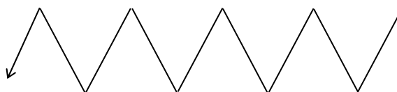
Figure 8. A chematic diagram of the arc wobble track of the cover layer
