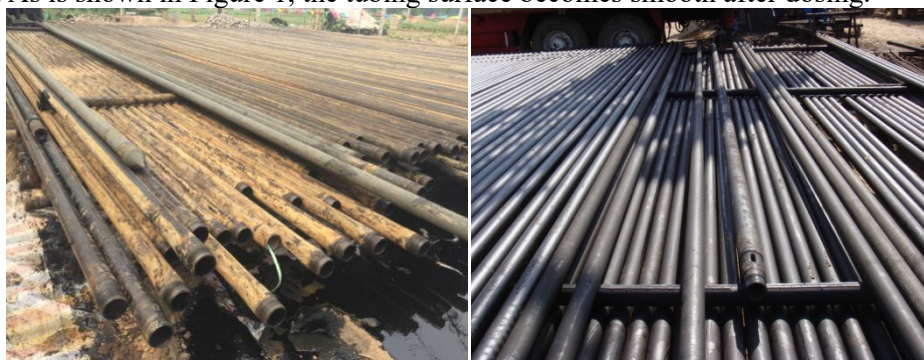
Fig.1 Comparison of corrosion morphology of pipes before and after adding medicine: a) before adding medicine, b) after adding medicine
