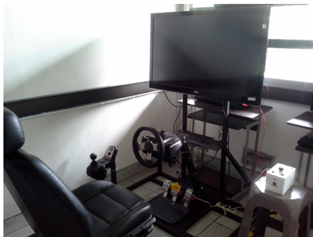
Figure 1. Driving simulator set.
