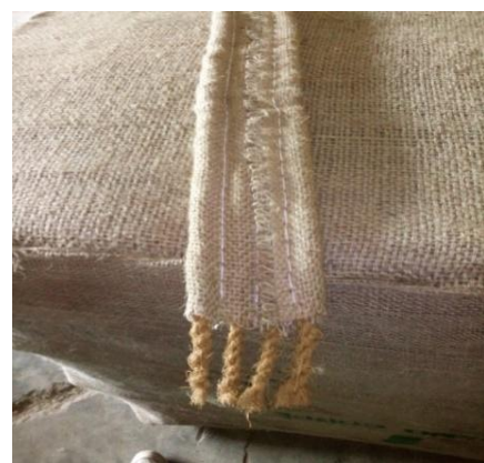
Figure 2. PVD material made of natural fibers
