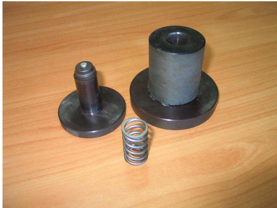
Figure 2. Device for springs contact predeformation.
