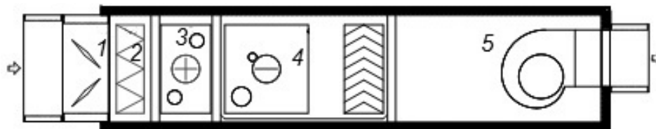
Figure 1. Standard setting of AHU-1 (CCFP-1.6-U3): 1 – front panel with valve, 2 – panel filter, 3 – hot-air heater, 4 – direct cooling air cooler, 5 – fan.
