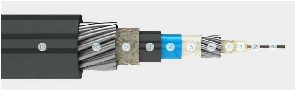
Figure 2. Cable type TPN2. 1 - optical fiber; 2- hydrophobic gel; 3- optical module; 4 - hydrophobic gel; 5 - iron wire armor; 6 - water-blocking tape; 7 - aluminopolymer tape; 8 - polyethylene sheath; 9 - hydrophobic gel; 10 - iron wire armor; 11 - polyethylene sheath.
