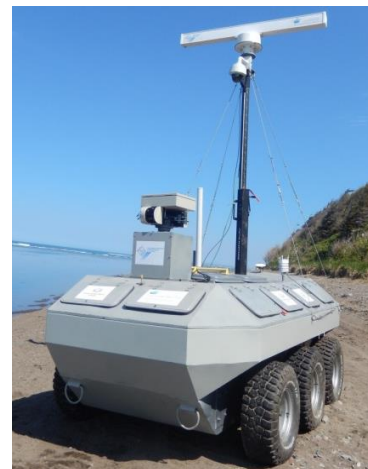
Figure 2. The special chassis for the movement in a coastal zone general view
