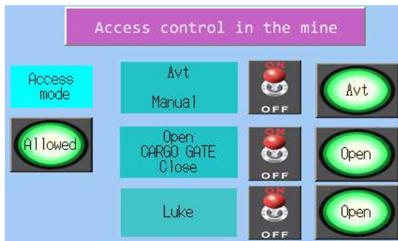
Figure 5. Structure of the dialog window to control the access system to the mine
