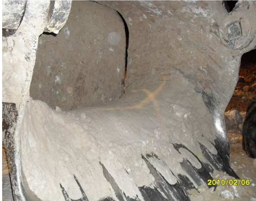
Figure 1. EKG-10 excavator bucket with frozen over soil (Korshunovski MCC).
