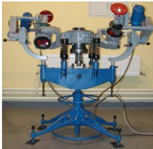
Figure 2. The laboratory prototype of the shock-vibration crusher with spatial motions of the active members.
