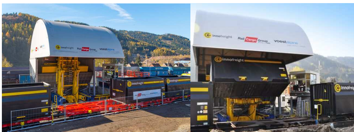
Figure 1. Unloading of open-top modules (containers) in the bunker by rotation
