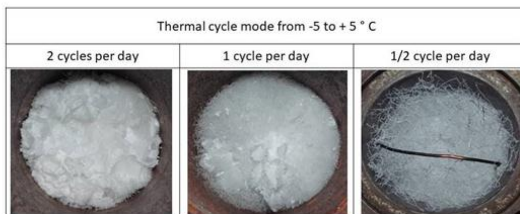
Figure 2. Images of the change in shapes of NGH depending on the thermal cycle of synthesis.
