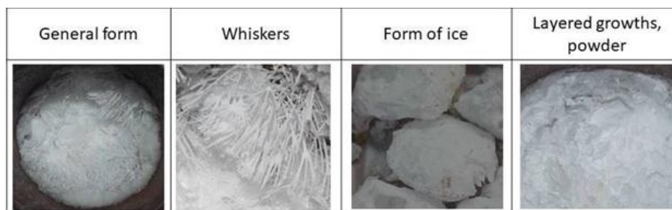
Figure 3. Images of various forms of NGH obtained from ice: whiskers, form of ice, powder and layered growths.
