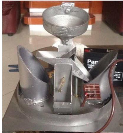
Figure 4. Tipping Bucket design for rain gauge measuring device
