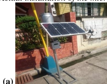
Figure 9. Testing Overall System with sensors for comparing the temperature, humidity and amount of rainfall (a) daytime and (b) night time
