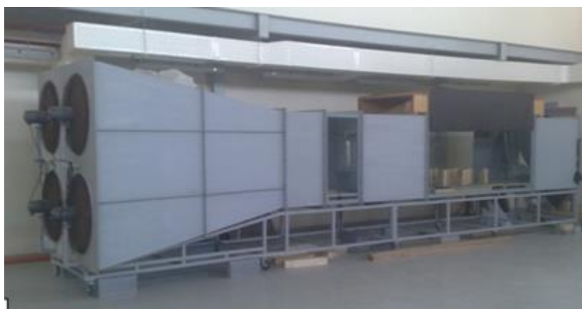
Figure 4. The environmental wind tunnel.
