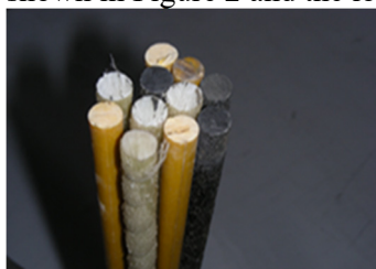
Figure 1. Thread shaped surface bonded sand CFRP bars, GFRP bars and plain GFRP bars
