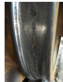
Figure 2. Wheel spalling
