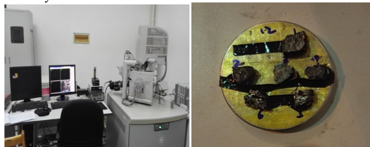
Fig.5 Quanta 200F FESEM and coal sample preparation
