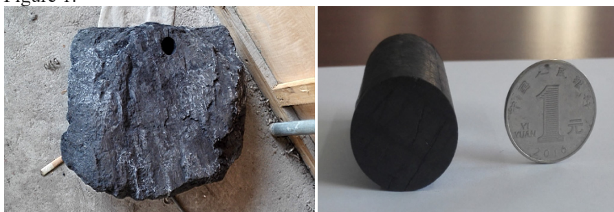
(a)Original coal rock sample map (b) Experimental Coal Heart Made by Wire Cutting Fig. 1 Samples of coal-rock in eastern Yunnan and western Guizhou
