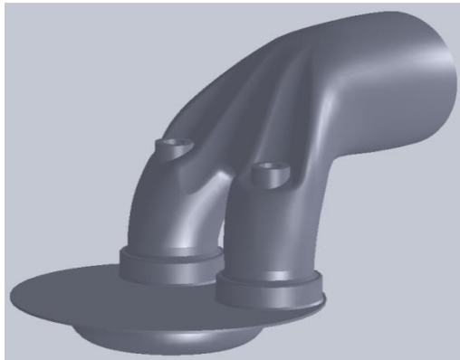
Figure. 7 The original intake port (1#).
