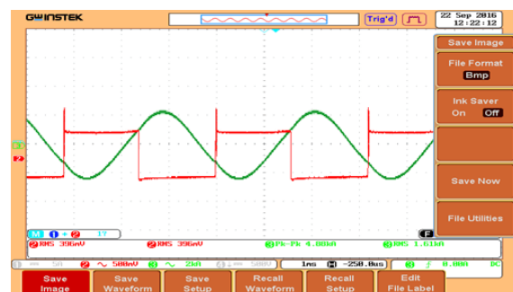
Figure 9. The current waveform of the resonant coil and the voltage waveform of the capacitor.
