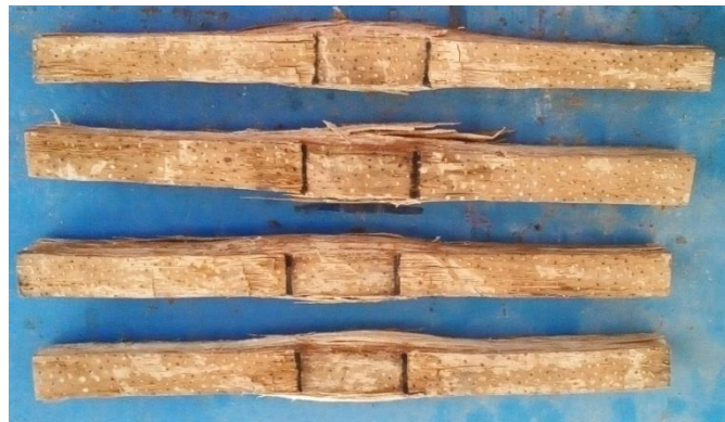
Figure 1. The form of sample damage after testing.
