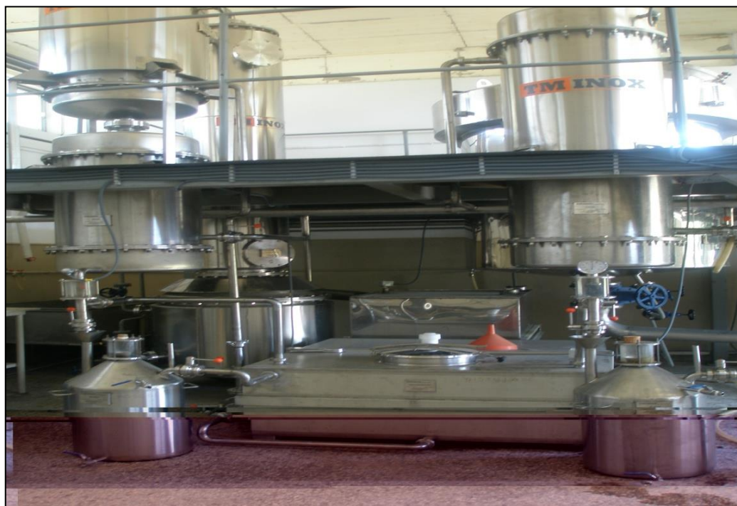
Figure 2. Presentation of the distillation process for the production of oregano essential oil.
