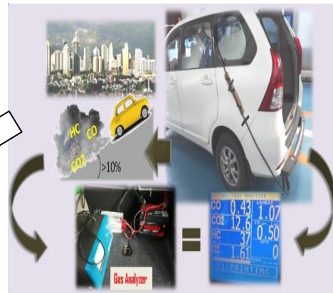
Figure 2. Setting up the gas analyzer CAP 320 on passenger cars with capacity 1300 cc.
