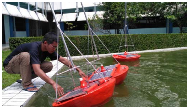
Figure 9. Stability and buoyancy test of the new AWCB in a pool at Fisheries and Marine Science Faculty, Bogor Agricultural University (IPB).
