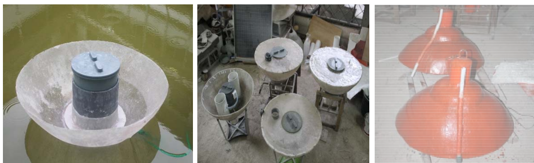
Figure 8. Process of buoy making. Uncovered buoy is floating in the freshwater (left), total molded buoy (center), coloring buoy (right).
