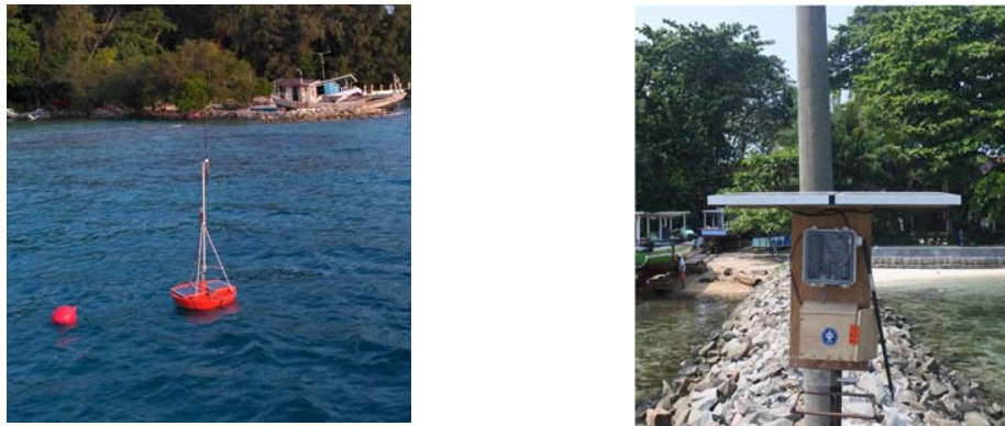
Figure 10. Field testing of aerial coastal buoys in surrounding waters of Pramuka Island, Node Buoy (left) and A Land-receiver (right).
