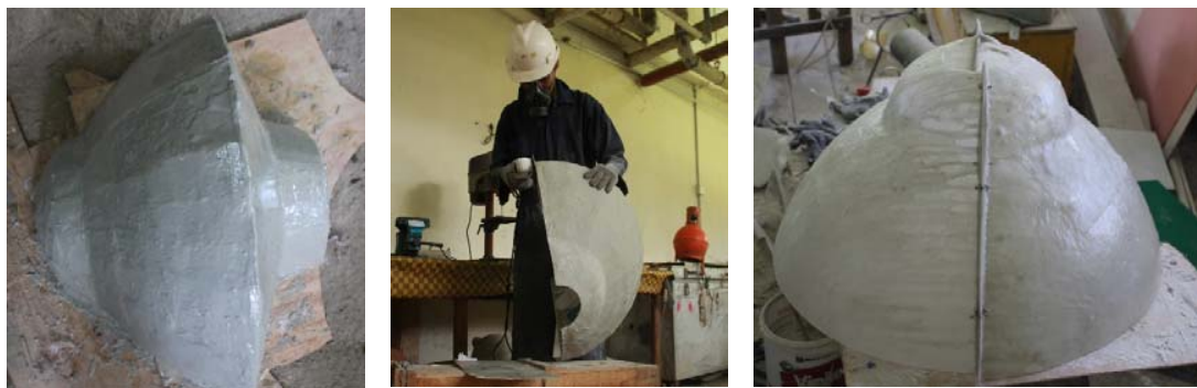
Figure 7. The buoy body's making process of Master (left), cleaning up the master (center) and set mold (right).
