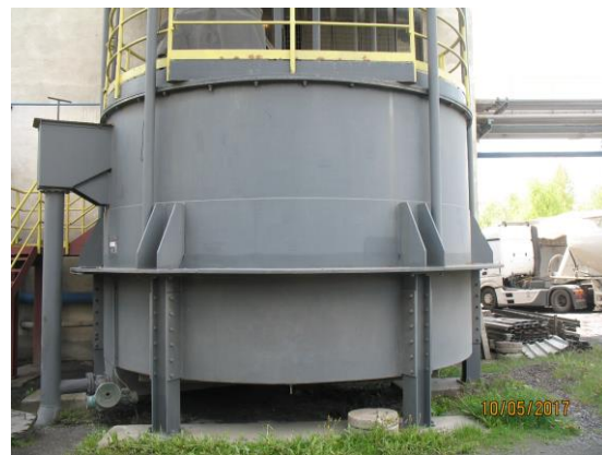
Figure 9. Hydromixture's retention tank.
