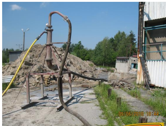
Figure 4. Flow mixer built-up in the field.
