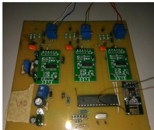
Figure 2: Strain gage bridge amplifiers on board with ADC, microcontroller and Wifi customised for datalogging.
