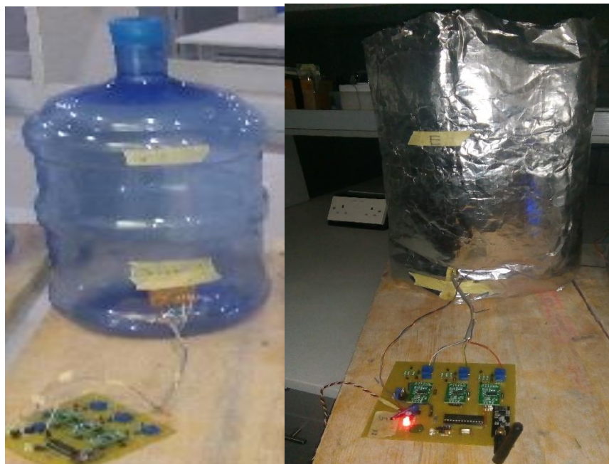
Figure 3: (LHS) Digester plastic before loading it with feedstocks. Attached to the lower side are the strain gages and temperature sensors which are connected to the data acquisition board. (RHS) Insulated digesters capped with tyre tube during data acquisition.
