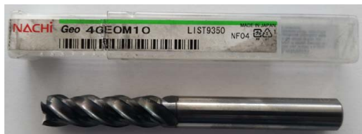
Figure 2. Carbide end mill, with \phi 10 mm diameter and 4 flutes
