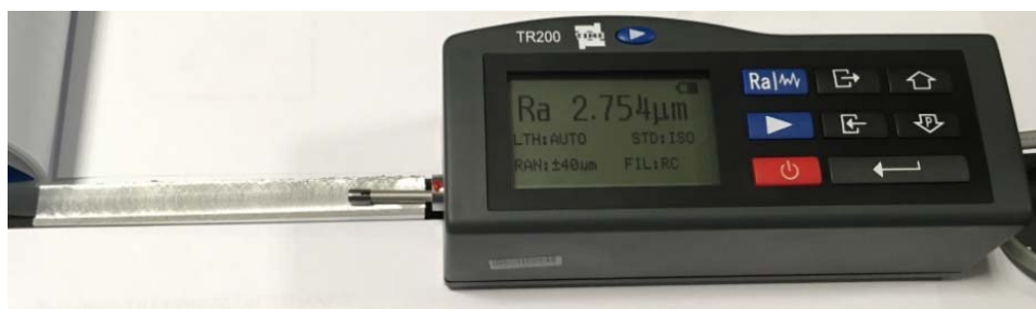
Figure 4. Portable surface roughness and workpiece
