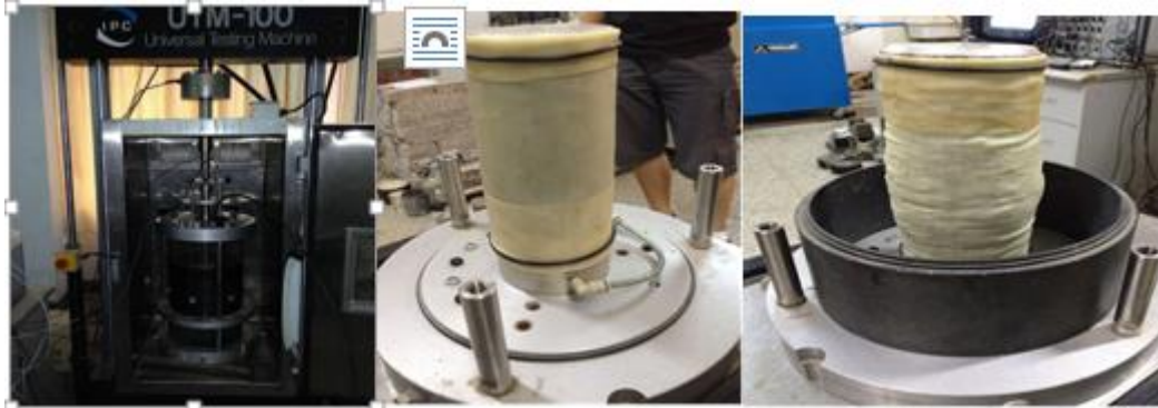
Figure 3.1 Forming and testing before and after test of three axis test
