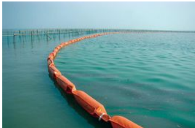
Figure 1. The containment boom
