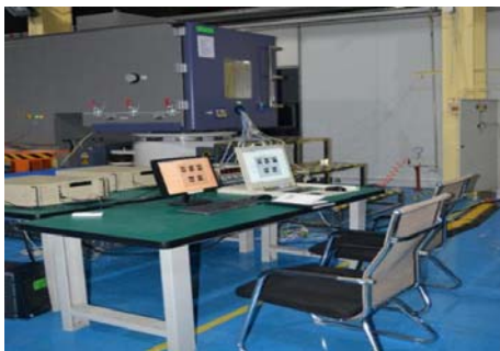
Figure 3. Accelerated degradation testing platform of Darlington transistor.
