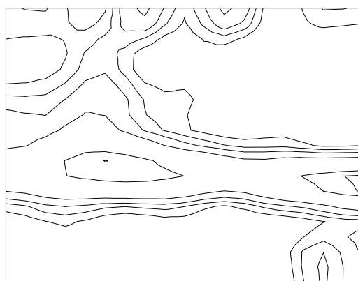
Fig 5. Sections of ODF at \phi_2=45^\circ (level: 1, 2, 4, 8, 10)
