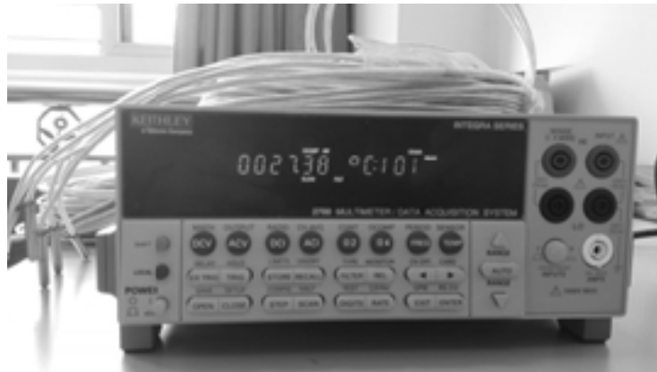
Figure 2. Keithley Model 2700 data acquisition system.
