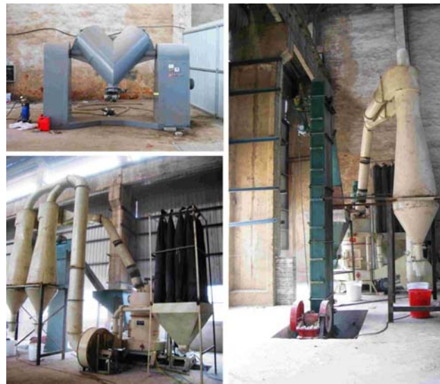
Figure 3. Whole-tailings paste backfilling material preparation system
