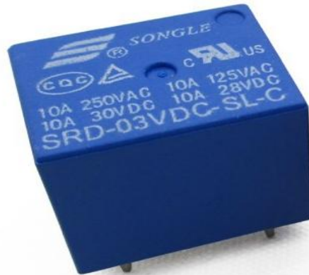
Figure 2. SRD-03VDC-SL-C relay used [25]
