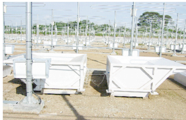
Figure 3. The hyperbolic horn speaker system at Kototabang. The speaker is mounted on a wooden frame with casters.
