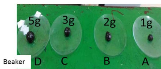
Figure 1. The weight of bio-gasification tar is varied. 1g, 2g, 3g, and 5g of bio-gasification tar is added in separate beakers A, B, C, and D respectively that contain 200 ml of ddH 2 O each.
