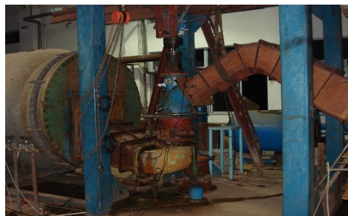
Figure 5. The experiment system of the axial-flow pump.
