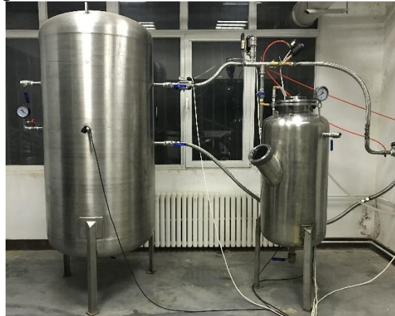
Figure 1. Observation tank and pressure control system
