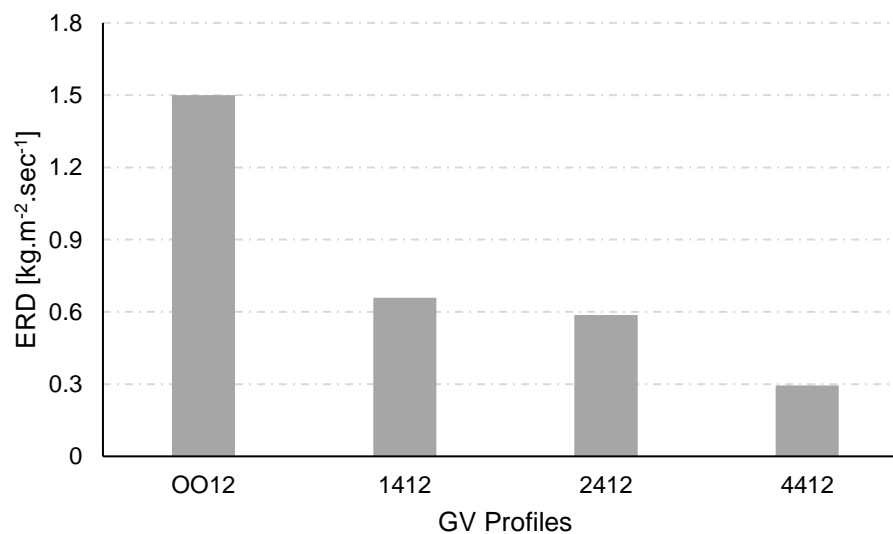
Figure 13. Erosion Rate Density for various Guide Vane Profile
