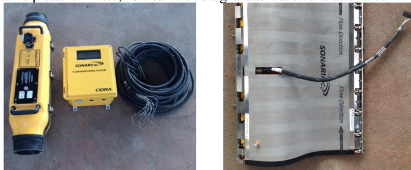
Figure 11. Sonar flowmeter
