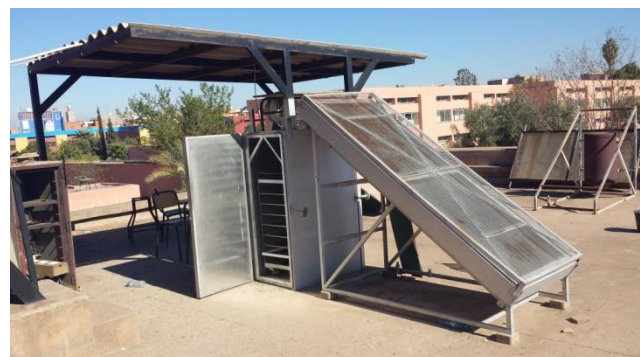
Figure. 1 Schematic diagram of the solar dryer: (1) Solar collector, (2) circulation fan, (3) fan, (4) air flow direction, (5) control box, (6) auxiliary heating system, (7) shelves, (8) drying chamber, (9) recycling air, (10) control foot, (11) exit of air, (12) humidity probes and (13) thermocouples
