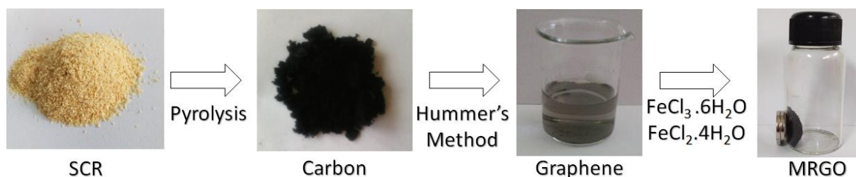
Figure 1. A schematic diagram of MRGO synthesis.
